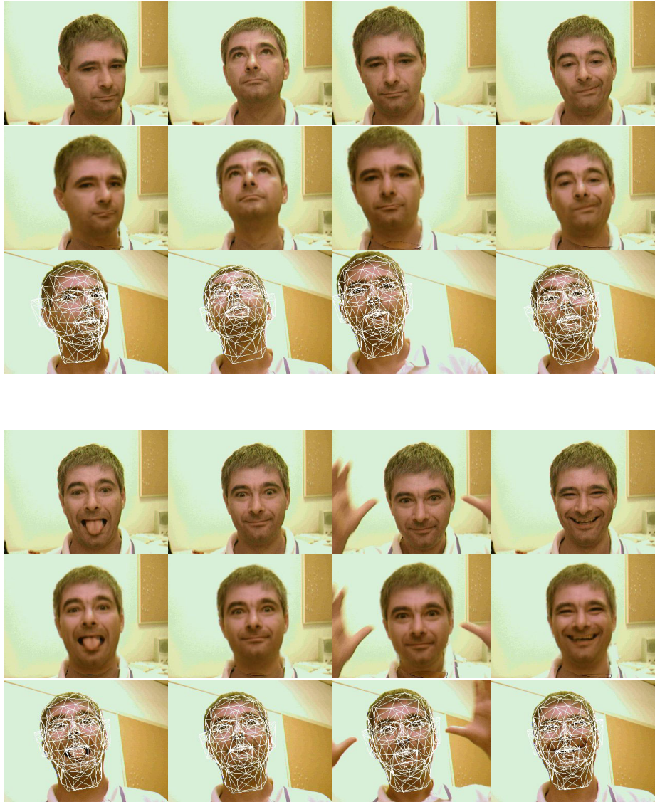
Fig. 7. Sample results from the second test sequence. The upper and lower rows are the original stereo images, while the middle rows are the synthesized ones. The triangular face model is overlaid on the bottom images. From left to right and from top to bottom, the frame numbers are 159, 200, 400, 577, 617, 720, 743, and 830.
